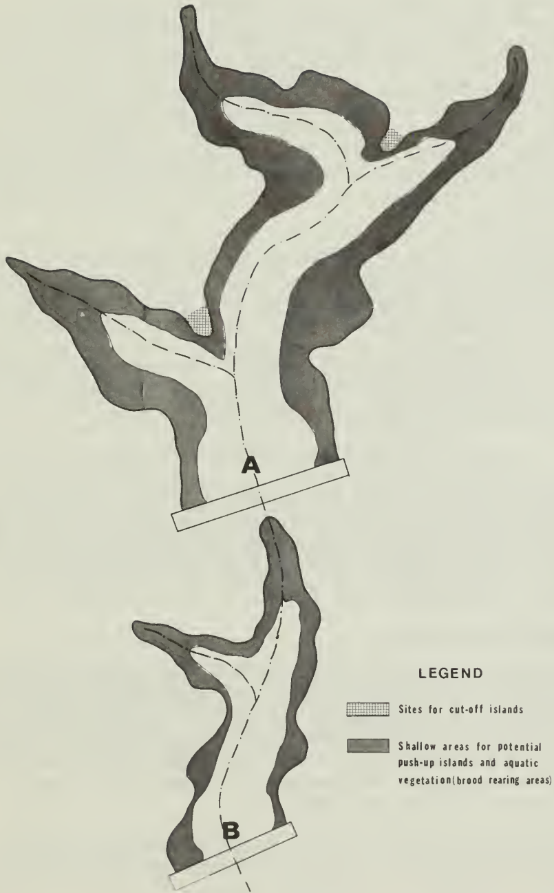
Figure 5. Potential sites for island construction in livestock reservoirs.
